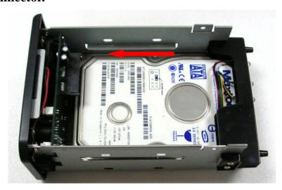
STEP3: Place the second HDD into the tray. Push the HDD to connect the SATA connector.
