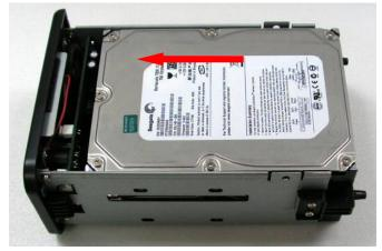
STEP4: Screw the HDD on the tray both sides.
