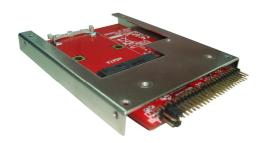
Best Solution that Easily Latch and Retain Fast Speed mSATA SSD as normally standard 7mm 2.5 inch IDE Drive!
